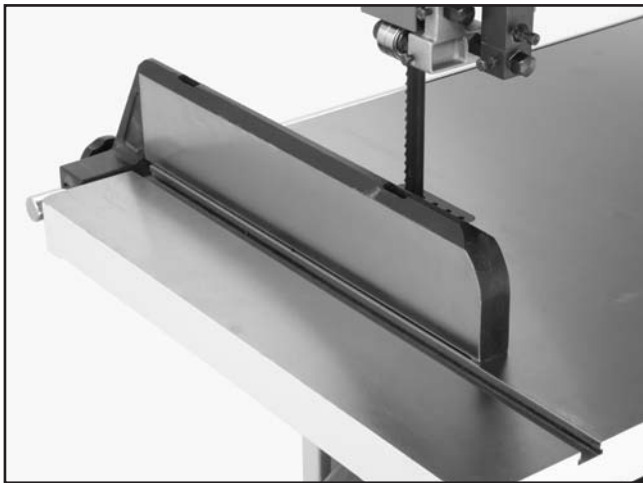
Figure 18. Fence square with miter slot.
